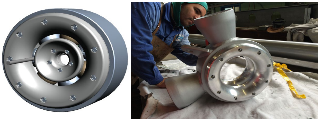
Figure 20 and 21: Simulation of the milled aluminium node and its realisation in workshop (Source F. Brogini)
