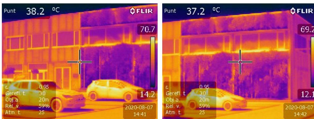
Figure 6. Infrared images of a vertical garden installed at SIOEN Ardoorie, which illustrates the temperatures differences measured between the cars, asphalt (55 - 67°C), the naked concrete wall (52 - 57°C), and the vertical garden (35 - 39 °C).
