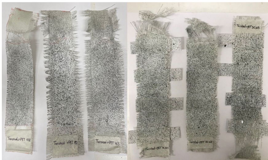
Figure 5. Sutex V2 Specimens after testing to failure. Regular specimens labelled “Twisted rPET W1-3” are referred to as “Sutex V2 W1-3” in this paper, and Solar Film specimens labelled “Twisted rPET SC W1-3” are referred to as “Sutex V2 SF W1-3” in this paper.
