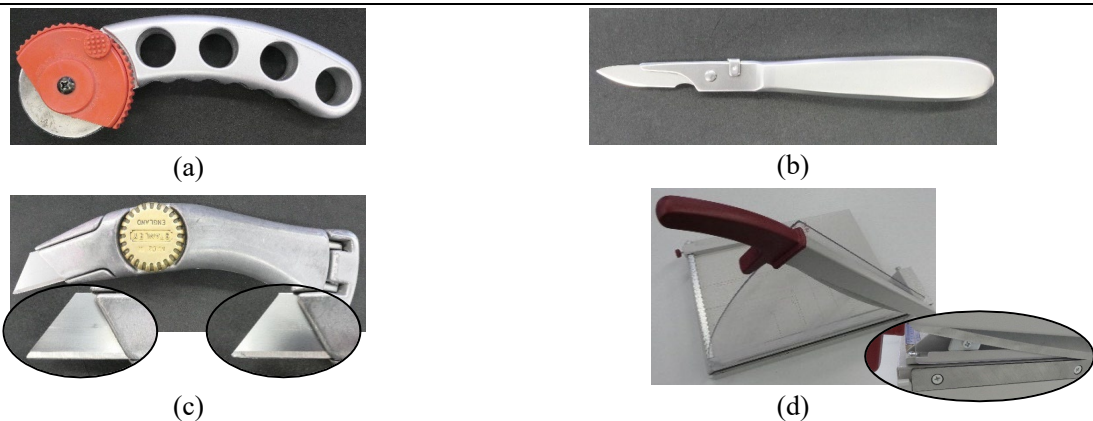
Figure 5: Investigated cutting tools; (a) rotary cutter; (b) scalpel with a new blade; (c) cutter knife with a new blade (left) and a used blade (right); (d) lever cutter
