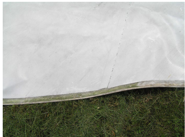
Figure 2b: PVC/PET fabric after 5 years
