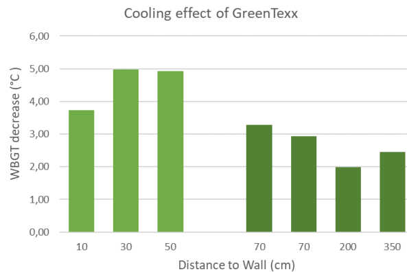
Figure 5. The WBGT decrease observed during the monitoring campaign at two locations (light and dark green) and across different distances (10 – 30 – 50 cm for the first vertical garden and 70 – 200 – 350cm for the second vertical garden).
