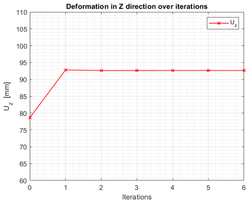
Figure 5: Deformation results in z direction of the central node vs. iteration steps
