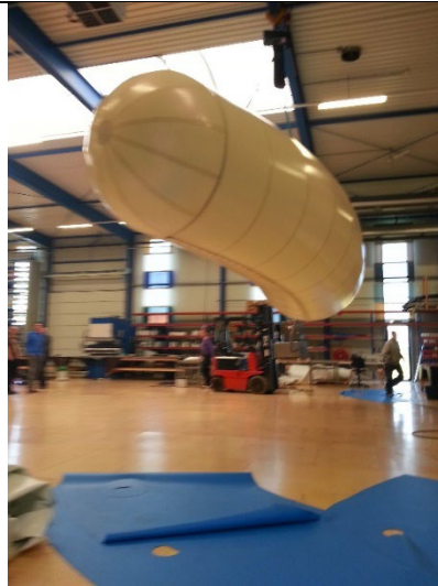
Figure 7: 1:1 mockup of a section part of the Tensairity outer ring
