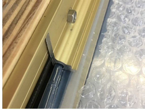
Figure 9: Fixation test of a clamping profile with inserted keder-pocket, ©Taiyo Europe
