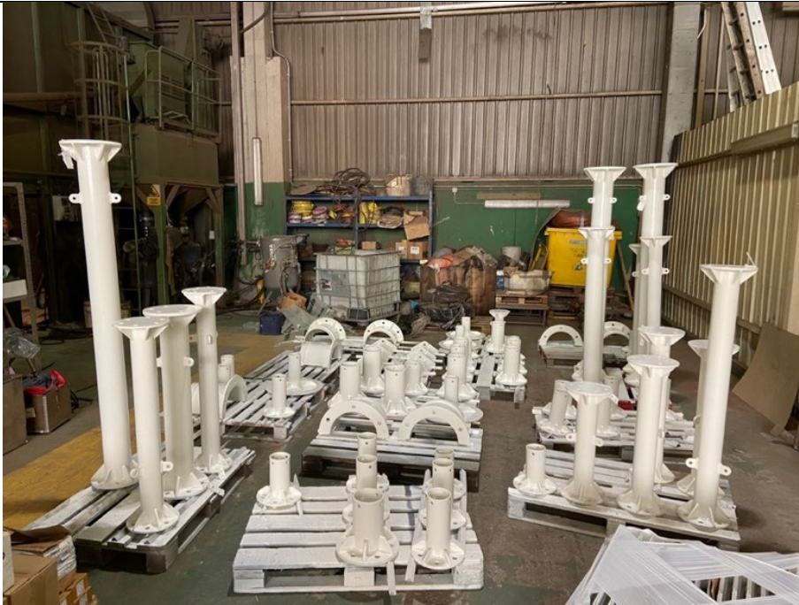
Figure 15 Steel floating masts elements sitting in the paint shop. The joints between shafts are all the same, but on different sizes.
