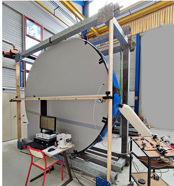
Figure 6: Experimental setup to measure the deflection of circular inflatable panels at various inflation and load levels.
