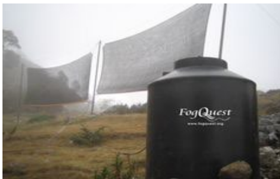
Figure 2: Large Fog Collector by Fog Quest
