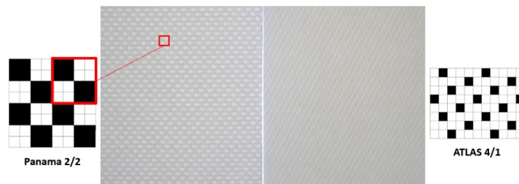
Figure 4: characteristics of ATLAS weave
